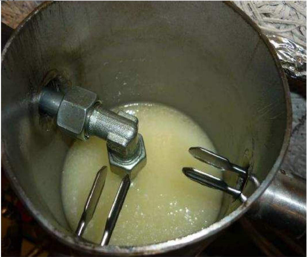
* Picture 10 : View details of fuel transport unit, into the open pre heater with the fill pipe (left) and the two level contacts
