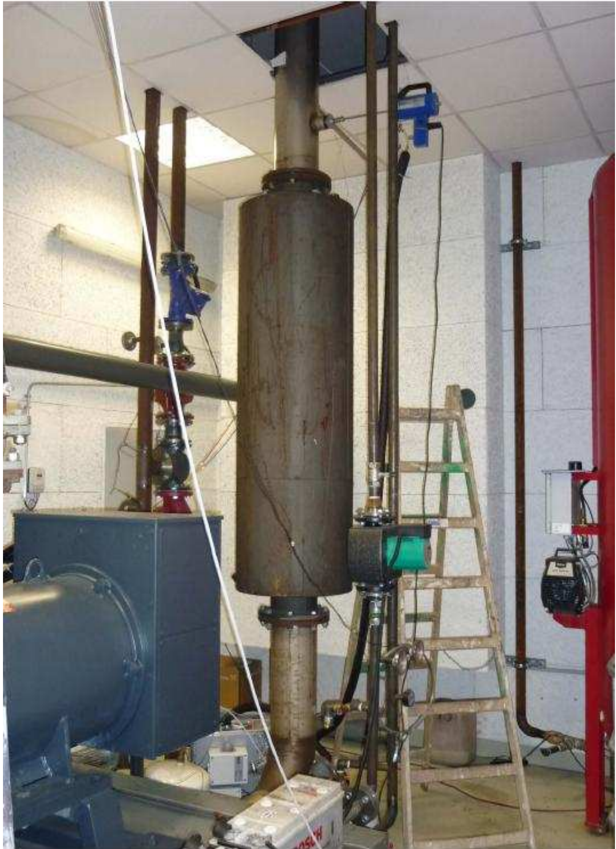
* Picture 14: sampling point for the continuous metering of air pollutant concentrations and exhaust flow
