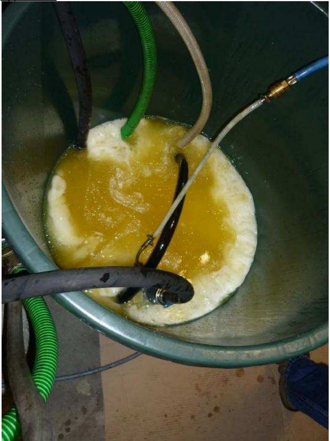
* Picture 5: beginning of the blending process of egm-fuel
