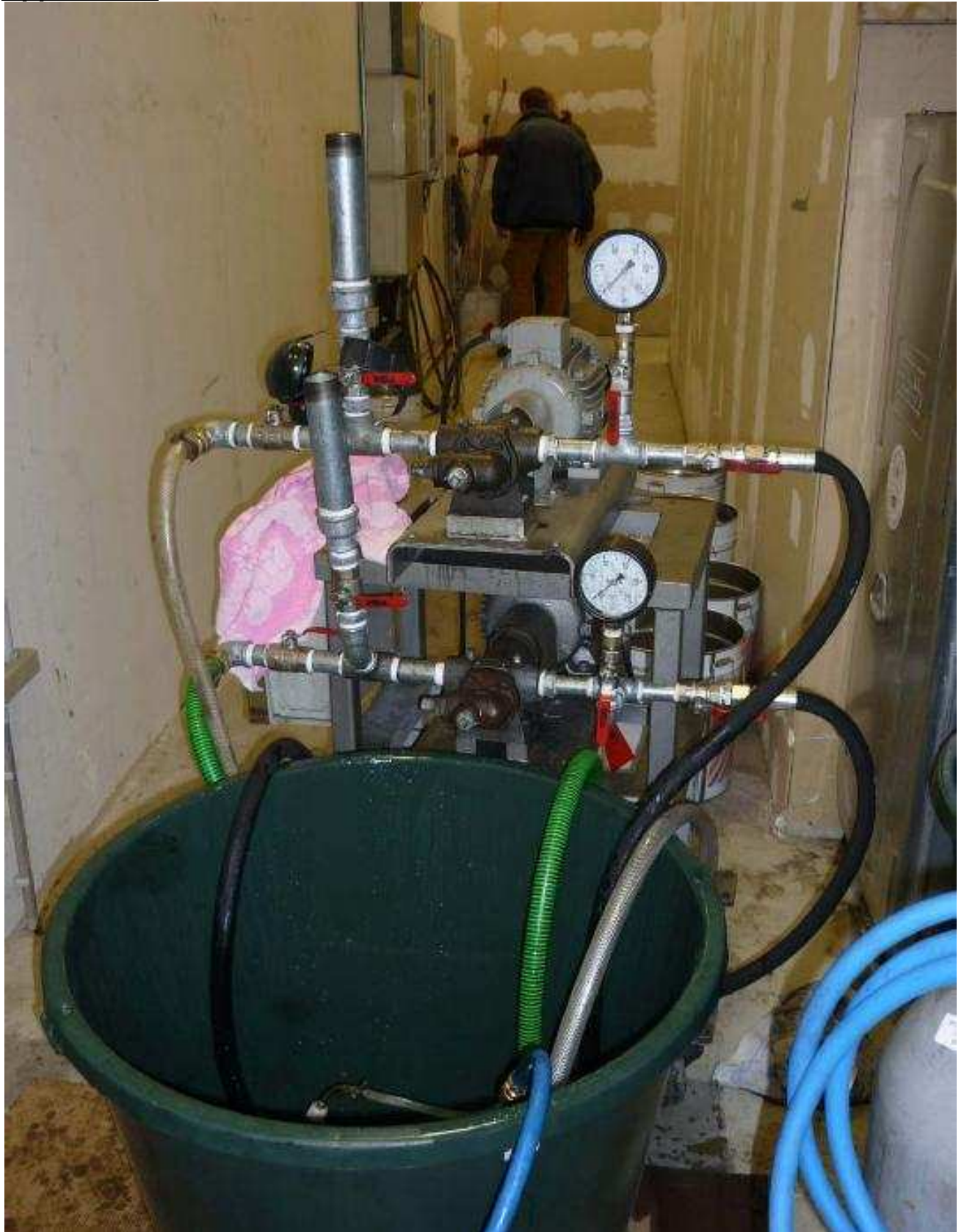
* Picture 3: Composite Drum with pump system for producing egm-fuel
